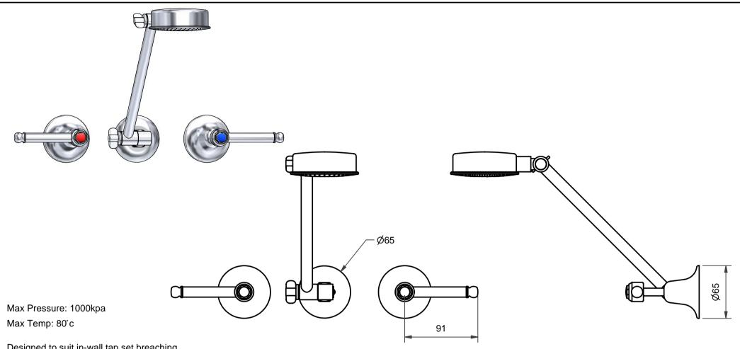
Designed to suit in-wall tap set breaching assemblies complying to AS 3718.
