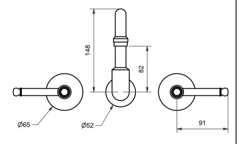
Designed to suit in-wall tap set breaching assemblies complying to AS 3718.
