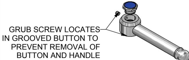
GRUB SCREW LOCATES IN GROOVED BUTTON TO PREVENT REMOVAL OF BUTTON AND HANDLE
