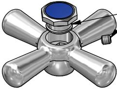
GRUB SCREW LOCATES IN GROOVED BUTTON TO PREVENT REMOVAL OF BUTTON AND HANDLE
