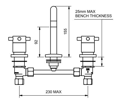
Headworks Available: Jumper Valve (Standard) Ceramic Disc 3/4 Turn (Optional)
