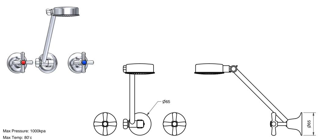
Designed to suit in-wall tap set breaching assemblies complying to AS 3718.
